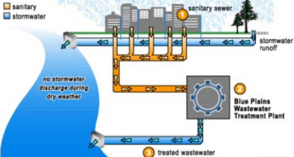
Separate Sanitary and Stormwater Sewer Systems
