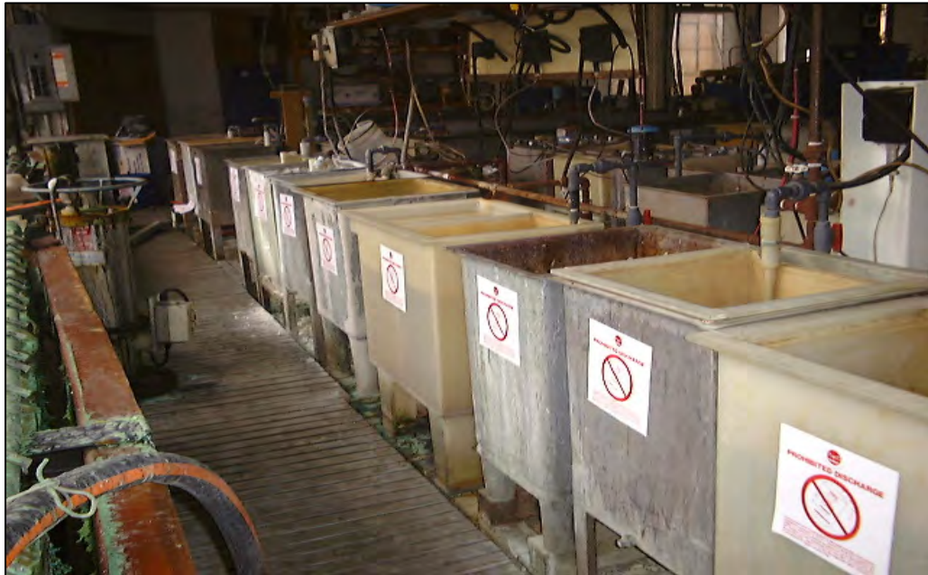
Tanks at a shutdown plating shop are stickered "PROHIBITED DISCHARGE"
