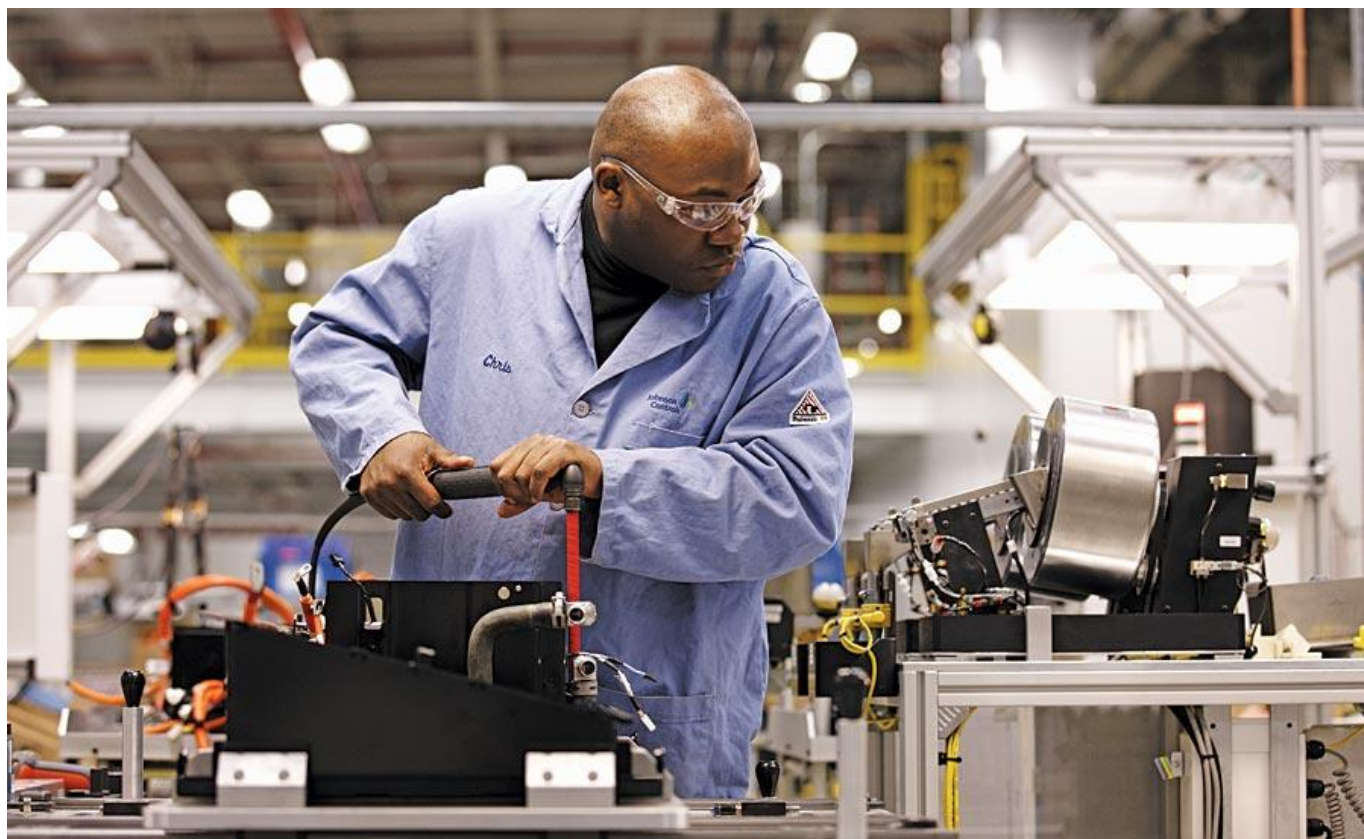
Johnson Controls' 12-volt Lithium-ion technology helps automakers to meet fuel efficiency and emissions regulations. Here, a worker assembles a li-ion battery pack at Johnson Controls' Holland, MI facility. Source: Johnson Controls
