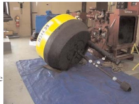
Painted Buoy with Sacrificial Anodes Installed
