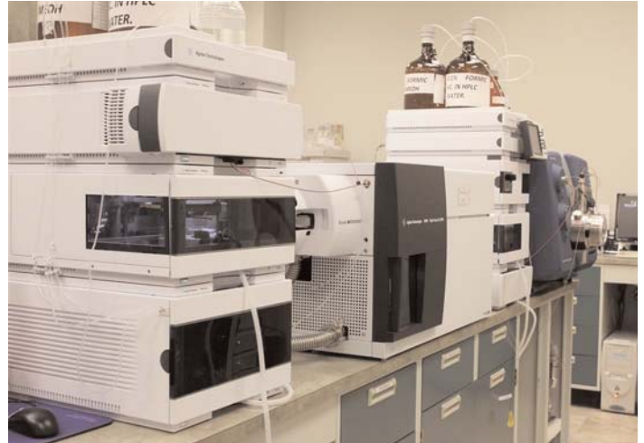
Example of the complex laboratory instrumentation required for PFAS sample analysis, including Ultra High Performance Liquid Chromatography-tandem Mass Spectrometry (courtesy of ADPEN Laboratories)
