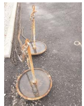
Buoy anchors and mooring chains undergoing annual inspection.
