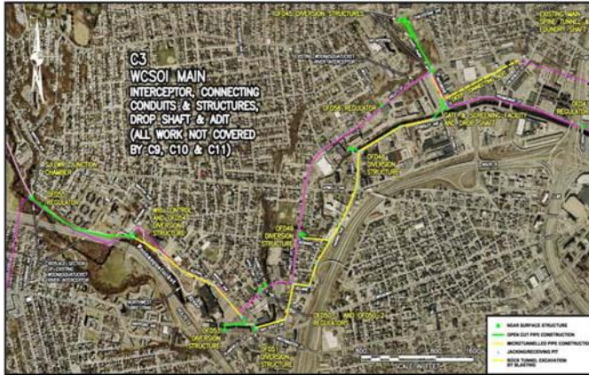
Photo: Proposed Woonasquatucket River CSO Interceptor Main alignment Project Overview
