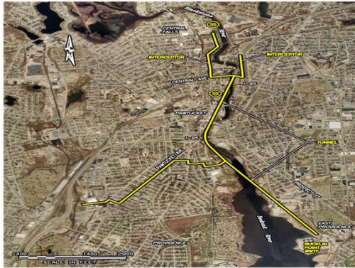
Photo: Proposed alignment for the Pawtucket CSO Tunnel
