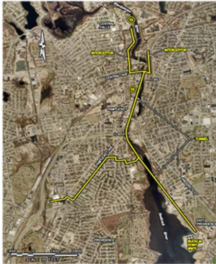
Photo: Alignment of CSO Phase III
