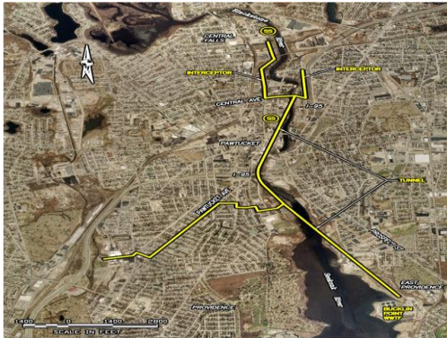
Photo: Proposed Phase III CSO Facilities
