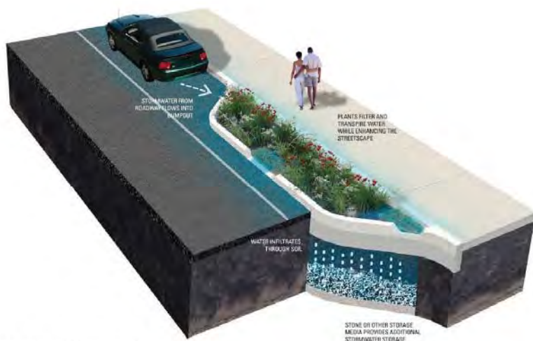
Mid-block Stormwater Bump-out
