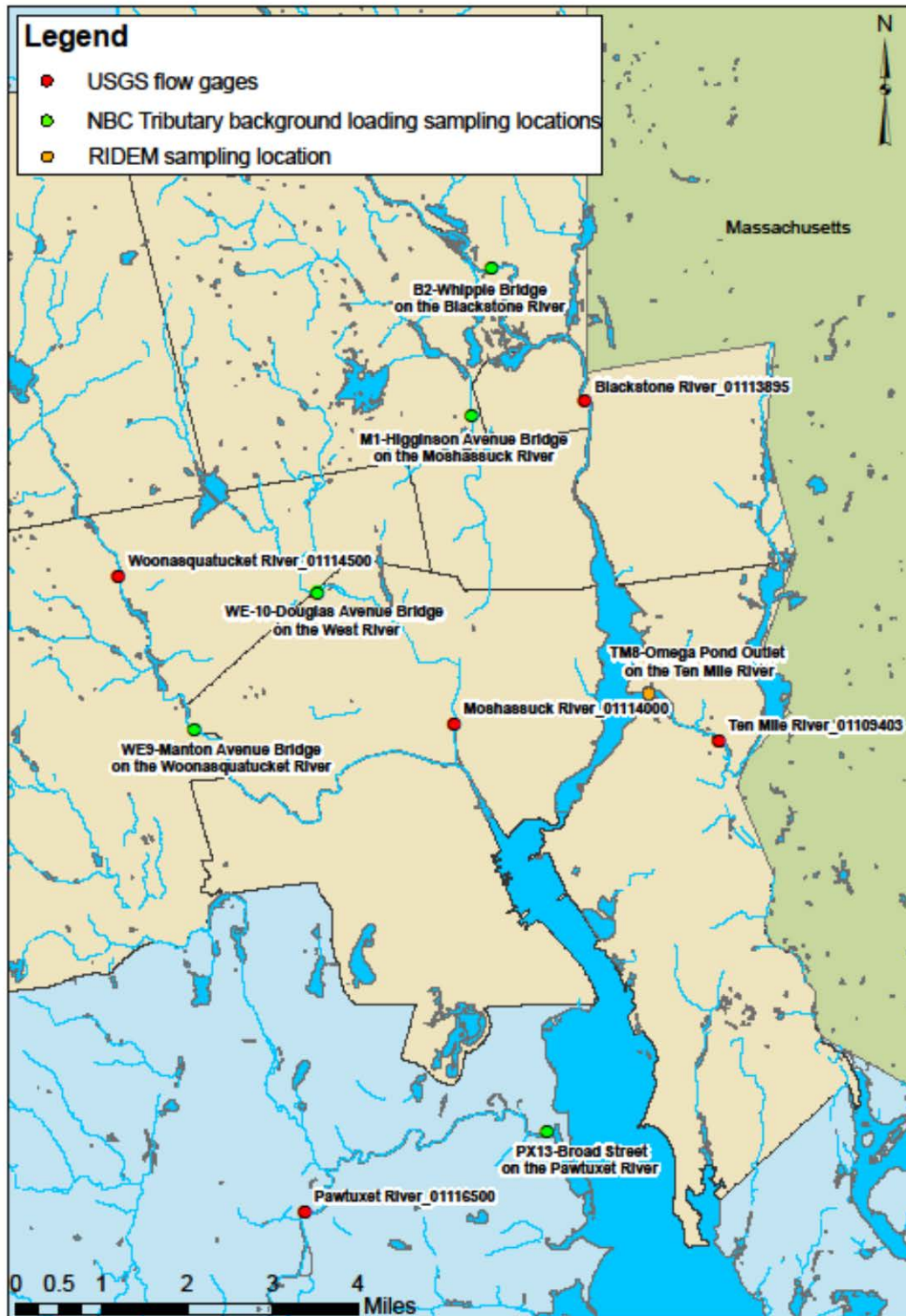
Figure 3-5. NBC sampling locations upstream of CSOs and USGS flow gauges used to calculate tributary FC background loadings
