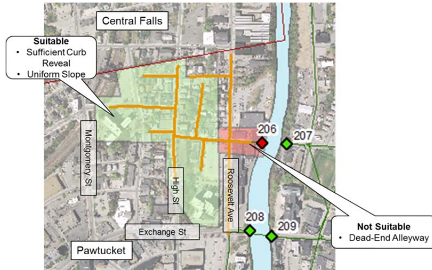
Figure 13 - Stormwater Management CSO 206
