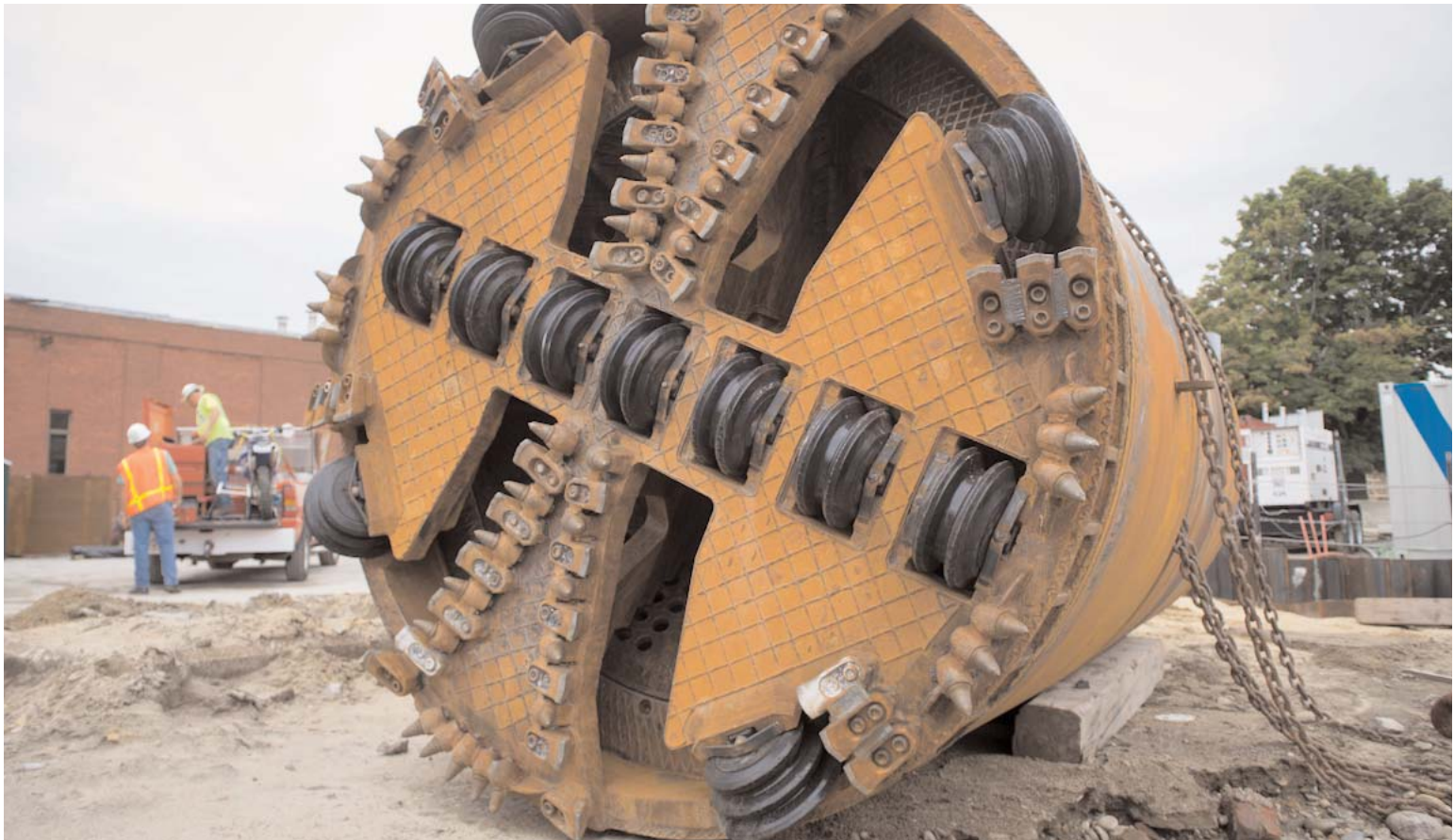
Above: A micro-tunneling machine on a rare visit above ground. This machine bores a tunnel thirty feet underground in which to place a new combined sewer overflow (CSO) interceptor, which can convey additional flow to the existing CSO tunnel.
