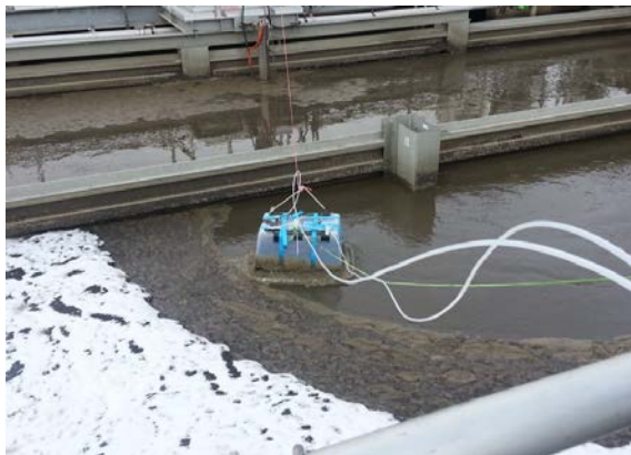
Photo: Green House Gas collection chamber deployed in treatment tank anoxic zone
