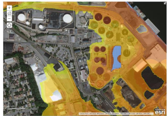
Using CRMC's StormTools application, this image shows how vulnerable NBC Field's Point property is to a 100-year coastal storm, resulting in 2-6 feet of water in various areas of the facility.
