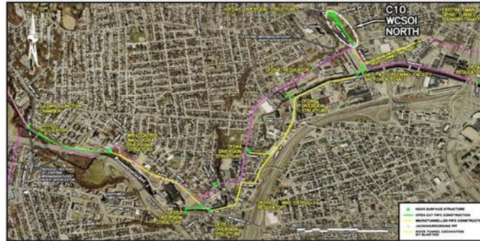
Photo: Proposed Woonasquatucket CSO Interceptor North alignment
