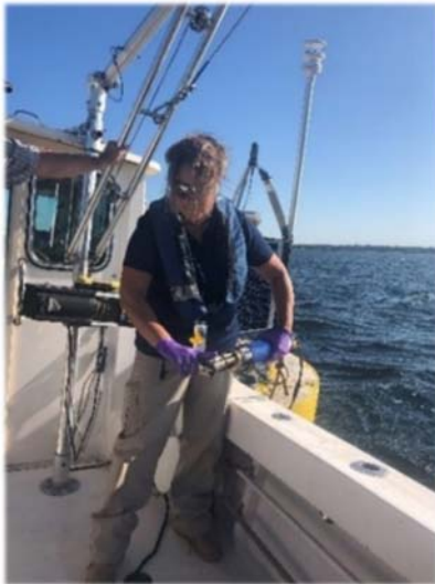
Photo: Environmental Monitoring staff replacing buoy sondes on Narragansett Bay
