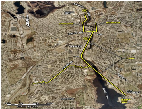
Photo: Proposed Phase III CSO Facilities
