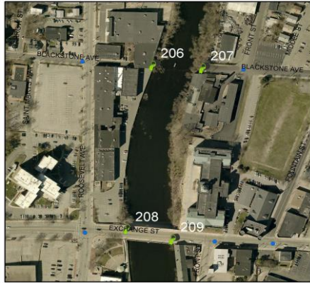
Photo: Outfall Locations
