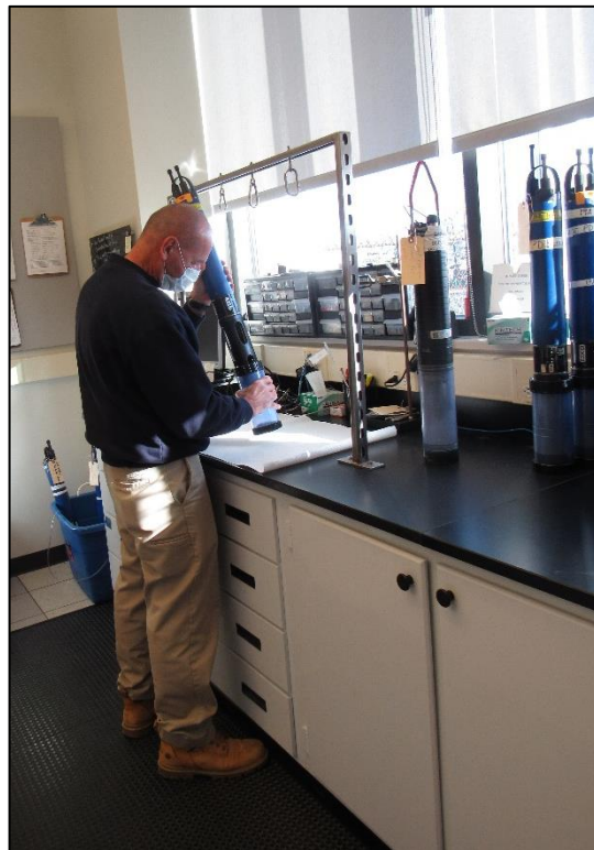
Environmental Monitoring staff calibrating sondes prior to deployment at a fixed-site station.
