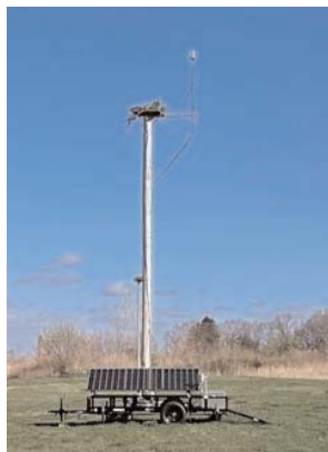
The osprey camera is powered by a portable photovoltaic system, built by BP Operations.
