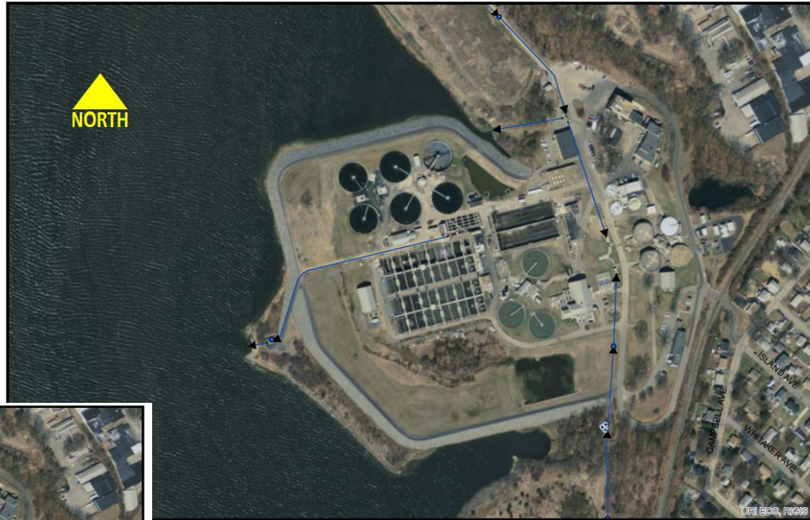
Narragansett Bay Commission Bucklin Point WWTF 2014 Photograph Showing 19.3 Foot (NGVD 1929) High Berm Constructed in 2012
