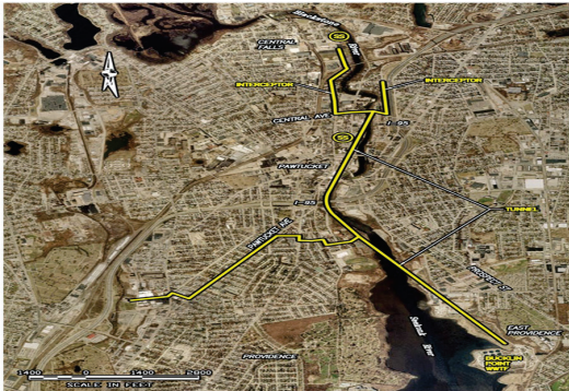
Photo: Proposed alignment for the Pawtucket CSO Tunnel
