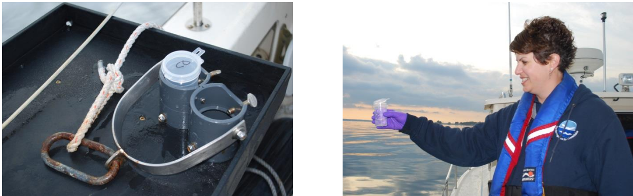
Figure 40. NBC fecal coliform sample collection device (left) and NBC staff collecting a bay fecal sample (right).
