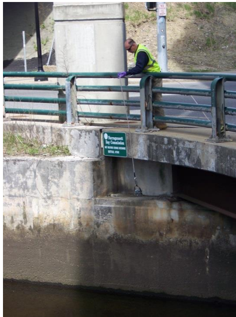
Figure 17. NBC staff collecting a river fecal coliform sample on the Woonasquatucket River near CSO 41.
