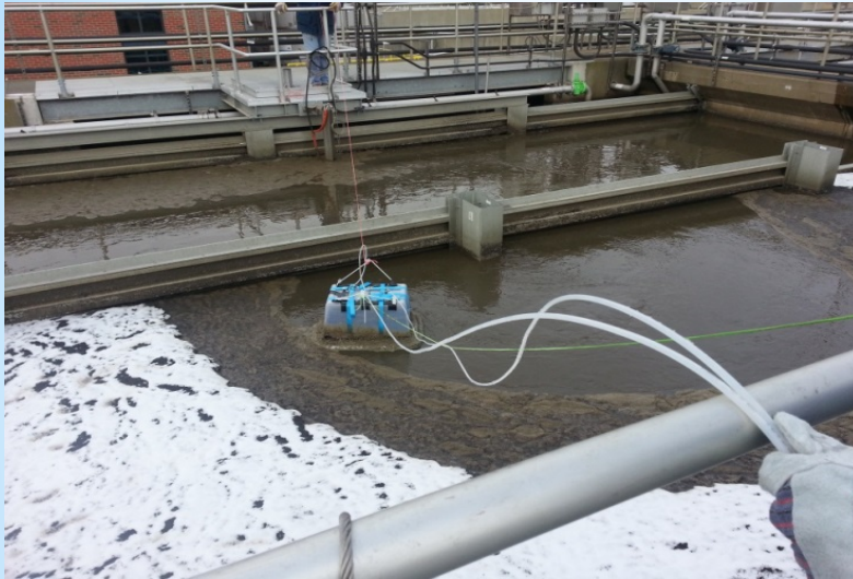
Floating chamber placed on water surface to measure GHG concentrations
