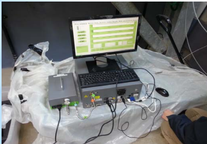
GHG analyzer that uses cavity ring down spectrometry to measure the ppm concentrations of GHGs: CO_2 , N_2O and CH_4
