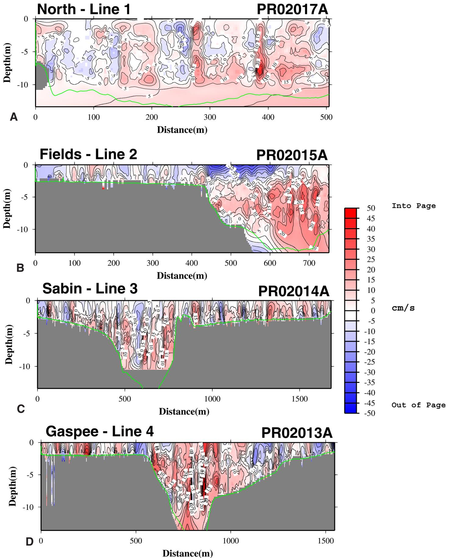
**Figure 4: Circuit 3 (early flood) velocity contours where values are projected normal to transect line. West is on the left, east is on the right, view is looking north. Red colors are flooding waters, or into the page, blue colors are ebbing waters, or flow out of the page. The green line marks the depth limit of reliable data.**
