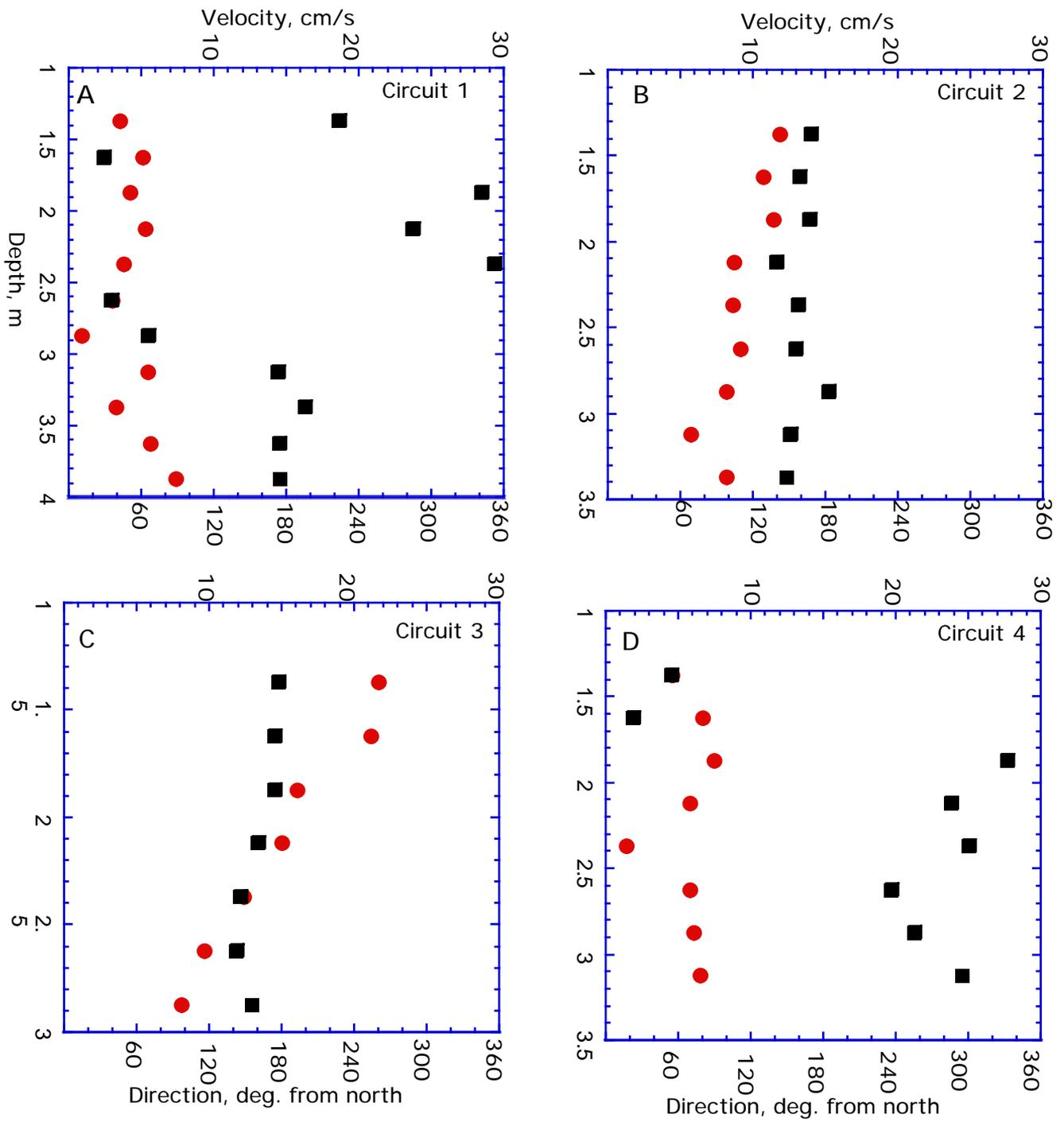
Figure 27: Velocity profiles obtained for transect 2, at the outfall, by holding position within the channel and collecting data for four minutes. Data have been averaged into a single profile of velocity versus depth. Shown are velocity magnitude (circles) and direction (squares), for each of the circuits; 1=early ebb, 2=mid-ebb, 3=late ebb and 4=early flood stages of the tide.
