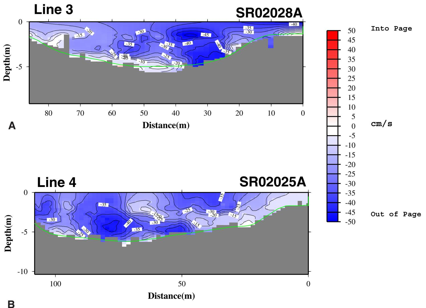
**Figure 24 : Circuit 3 (late ebb) velocity contours for Seekonk River Survey. Data are projected normal to transect lines. Lines are oriented roughly west(left) to east(right), with the view looking north. Red colors are flooding waters, or flow into the page, and blues are ebbing water, or flow out of the page. The green line marks the depth limit of reliable data.**
