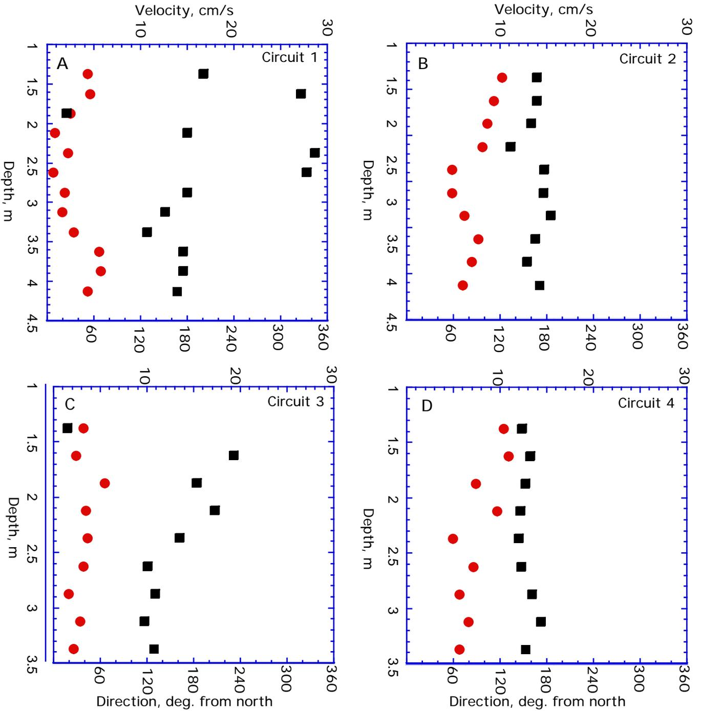
Figure 26: Velocity profiles obtained for transect 1 , northernmost line, by holding position within the channel and collecting data for four minutes. Data have been averaged into a single profile of velocity versus depth. Shown are velocity magnitude (circles) and direction (squares), for each of the circuits; 1=early ebb, 2=mid-ebb, 3=late ebb and 4=early flood stages of the tide.
