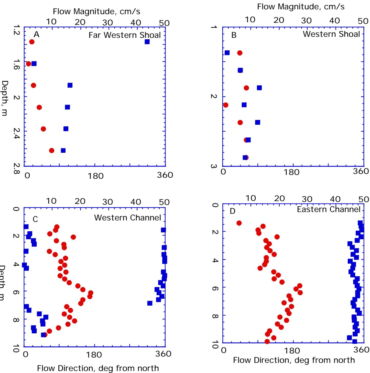
Figure 13: Laterally averaged velocity profiles for subsections of transect line 2, Fields Pt. Data are velocity magnitude (CIRCLES) and direction (SQUARES). The subsections include shallow regions to the west of the channel, and two subsections of the channel. The tidal stage is CIRCUIT 4, or late flood conditions.
