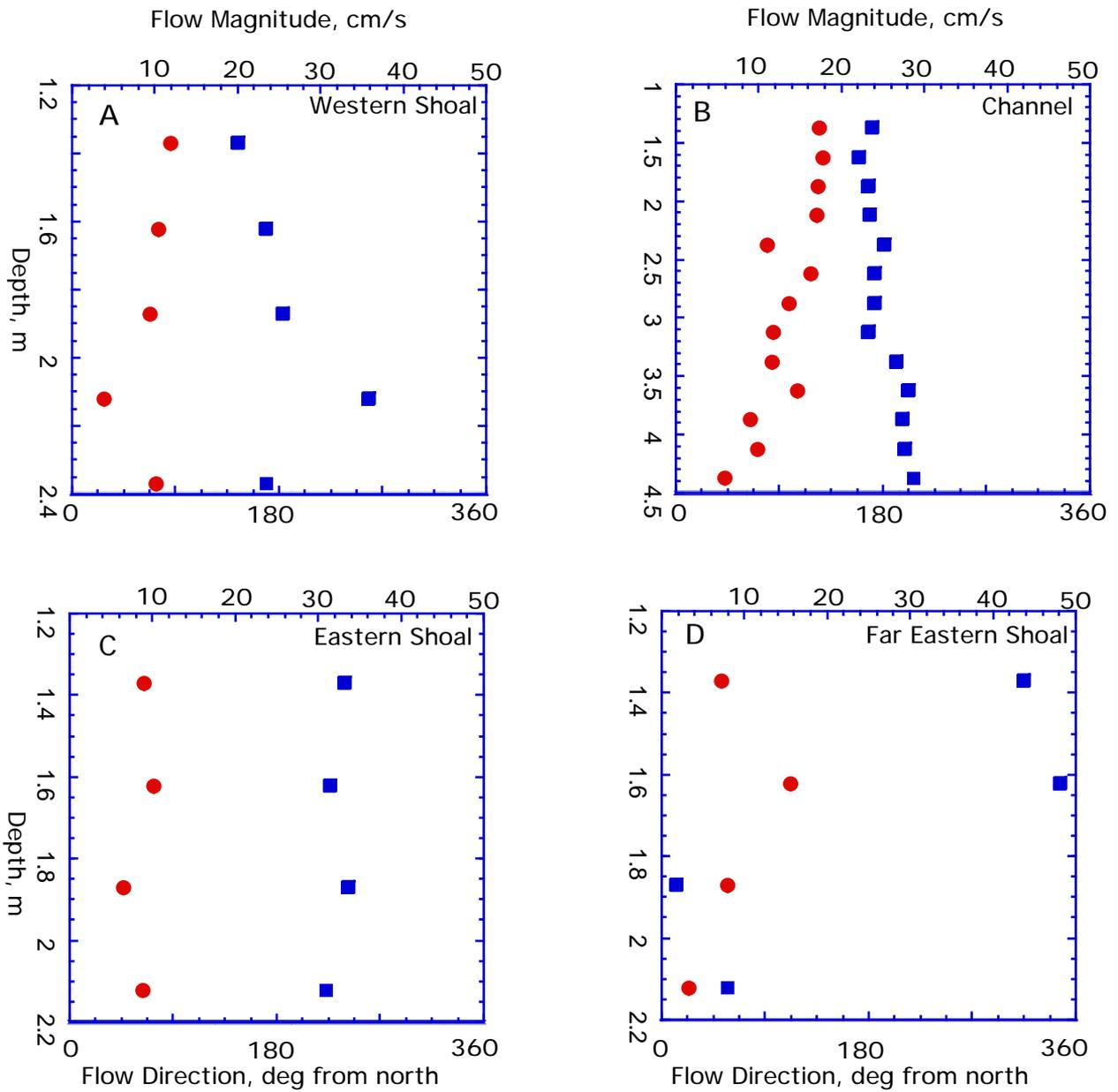
Figure 17: Laterally averaged velocity profiles for subsections of transect line 3, Sabin Pt. Data are velocity magnitude (CIRCLES) and direction (SQUARES). The subsections include shallow regions to the east and west of the channel, and the channel. The tidal stage is CIRCUIT 2, or late ebb conditions.
