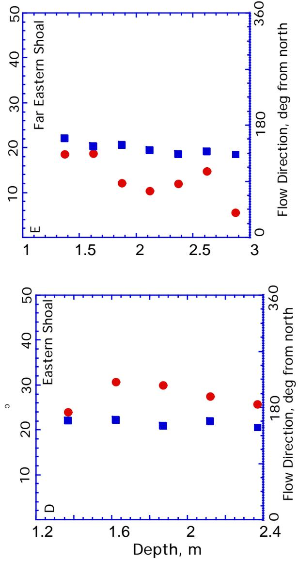
Figure 16: Laterally averaged velocity profiles for subsections of transect line 3, Sabin Pt. Data are velocity magnitude (CIRCLES) and direction (SQUARES). The subsections include shallow regions to the east and west of the channel, and the channel. The tidal stage is CIRCUIT 1, or ebb conditions.
