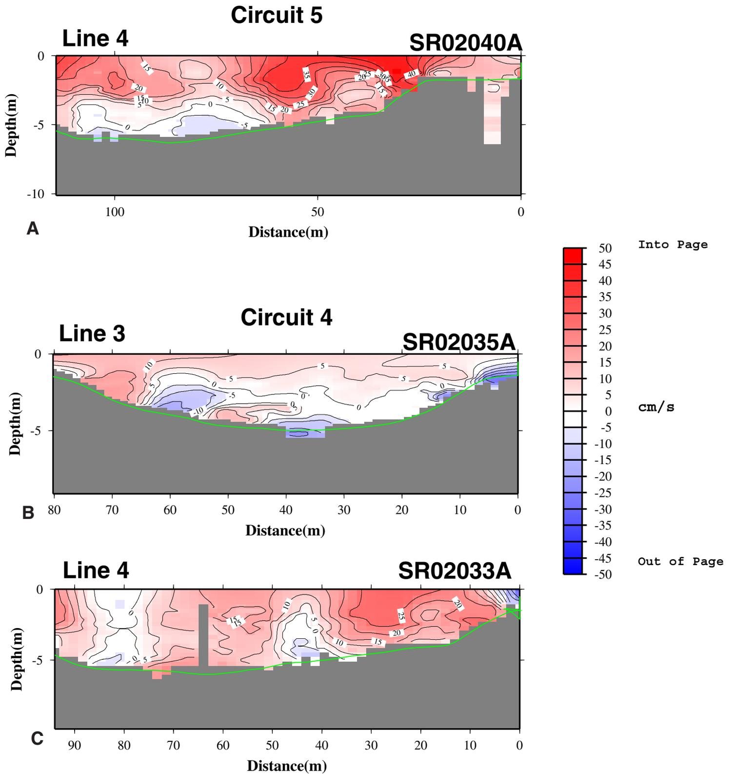
**Figure 25 : Plots of transect normal velocity data from Circuits 4 (early flood) and 5 (mid-flood) of the Seekonk River survey. Cross channel transects were only driven on lines 3 and 4 during this stage of the tide.**
