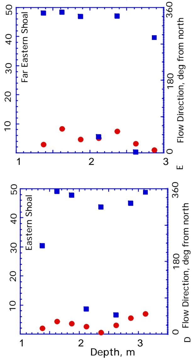
Figure 19: Laterally averaged velocity profiles for subsections of transect line 3, Sabin Pt. Data are velocity magnitude (CIRCLES) and direction (SQUARES). The subsections include shallow regions to the east and west of the channel, and the channel. The tidal stage is CIRCUIT 4, or late flood conditions.
