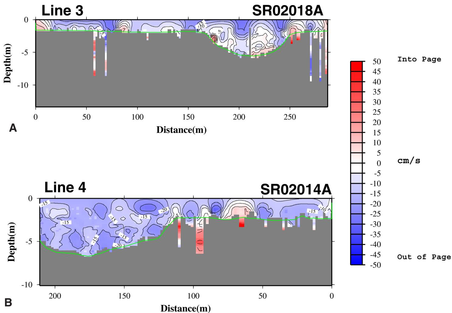
**Figure 23 : Circuit 2 (mid-ebb) velocity contours for Seekonk River Survey. Data are projected normal to transect lines. Lines are oriented roughly west(left) to east(right), with the view looking north. Red colors are flooding waters, or flow into the page, and blues are ebbing water, or flow out of the page. The green line marks the depth limit of reliable data.**
