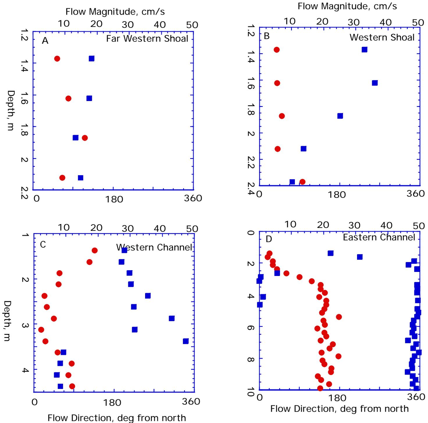
Figure 12: Laterally averaged velocity profiles for subsections of transect line 2, Fields Pt. Data are velocity magnitude (CIRCLES) and direction (SQUARES). The subsections include shallow regions to the west of the channel, and two subsections of the channel. The tidal stage is CIRCUIT 3, or early flood conditions.
