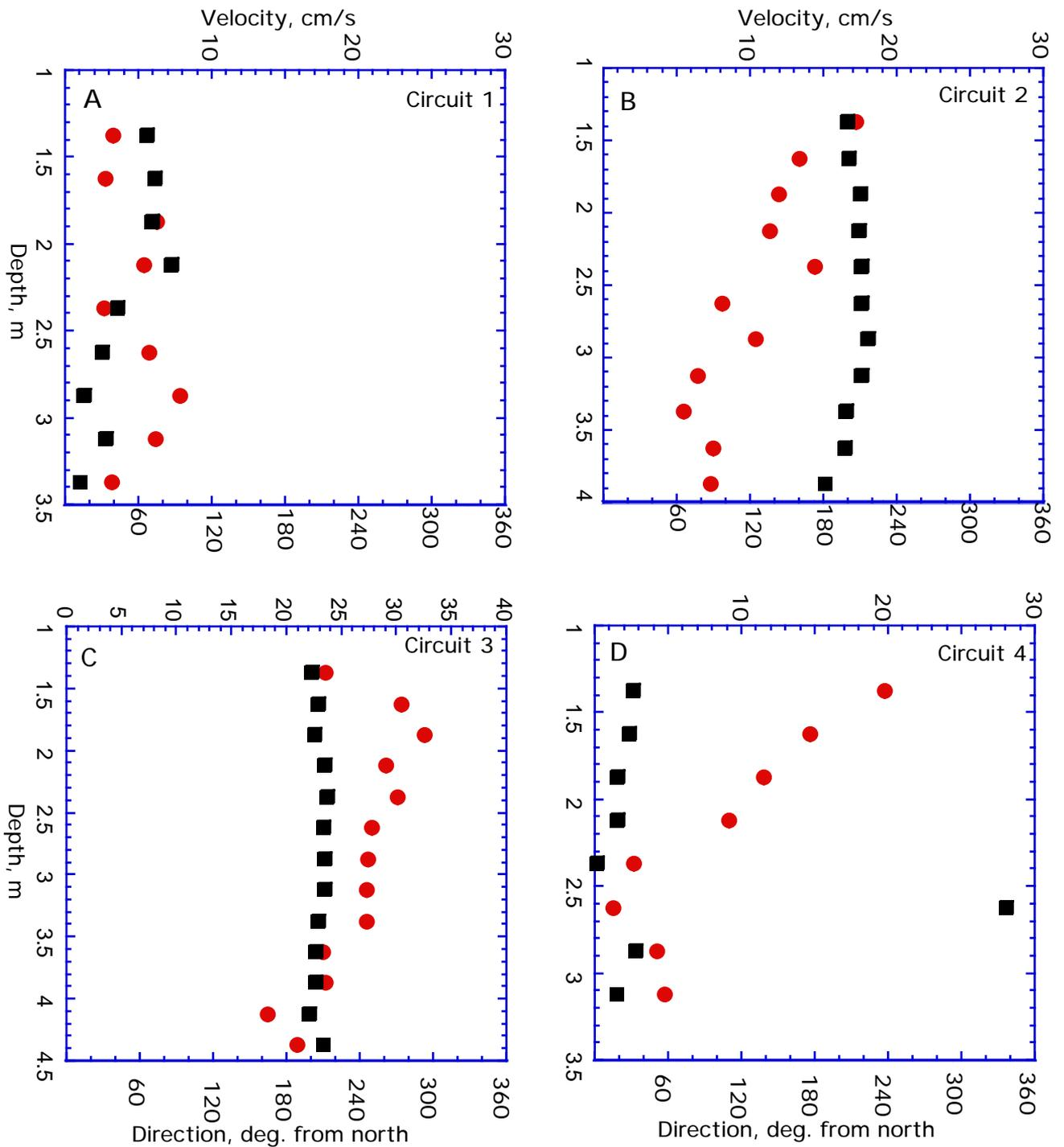
Figure 29: Velocity profiles obtained for transect 3 by holding position within the channel and collecting data for four minutes. Data have been averaged into a single profile of velocity versus depth. Shown are velocity magnitude (circles) and direction (squares). Time periods are circuits 1, 2 and 3 or early, mid and late ebb conditions. Circuit 4 is early flood.
