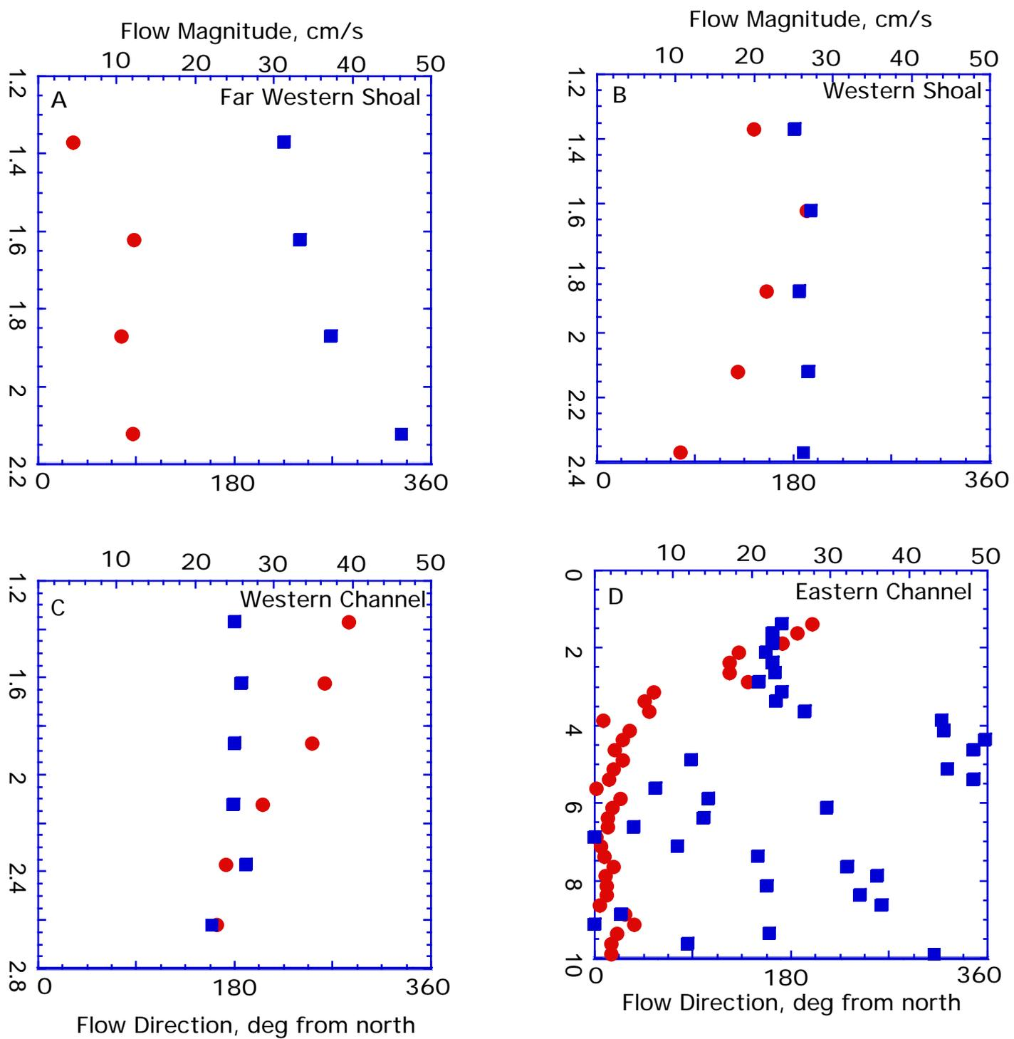
Figure 10: Laterally averaged velocity profiles for subsections of transect line 2, Fields Pt. Data are velocity magnitude (CIRCLES) and direction (SQUARES). The subsections include shallow regions to the west of the channel, and two subsections of the channel. The tidal stage is CIRCUIT 1, or ebb conditions.
