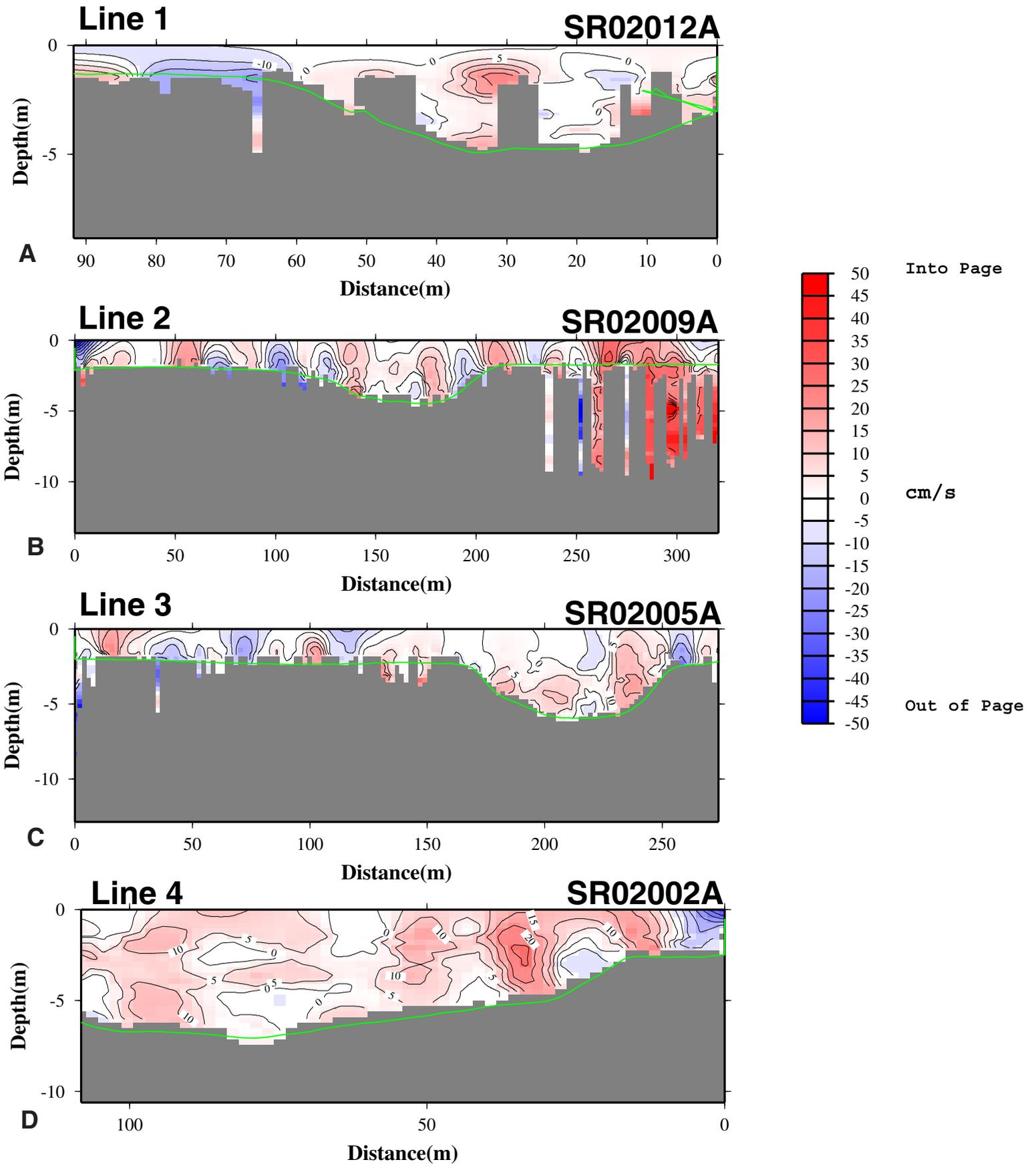
**Figure 22 : Circuit 1 (early ebb) velocity contours for Seekonk River Survey. Data are projected normal to transect lines. Lines are oriented roughly west(left) to east(right), with the view looking north. Red colors are flooding waters, or flow into the page, and blues are ebbing water, or flow out of the page. The green line marks the depth limit of reliable data.**
