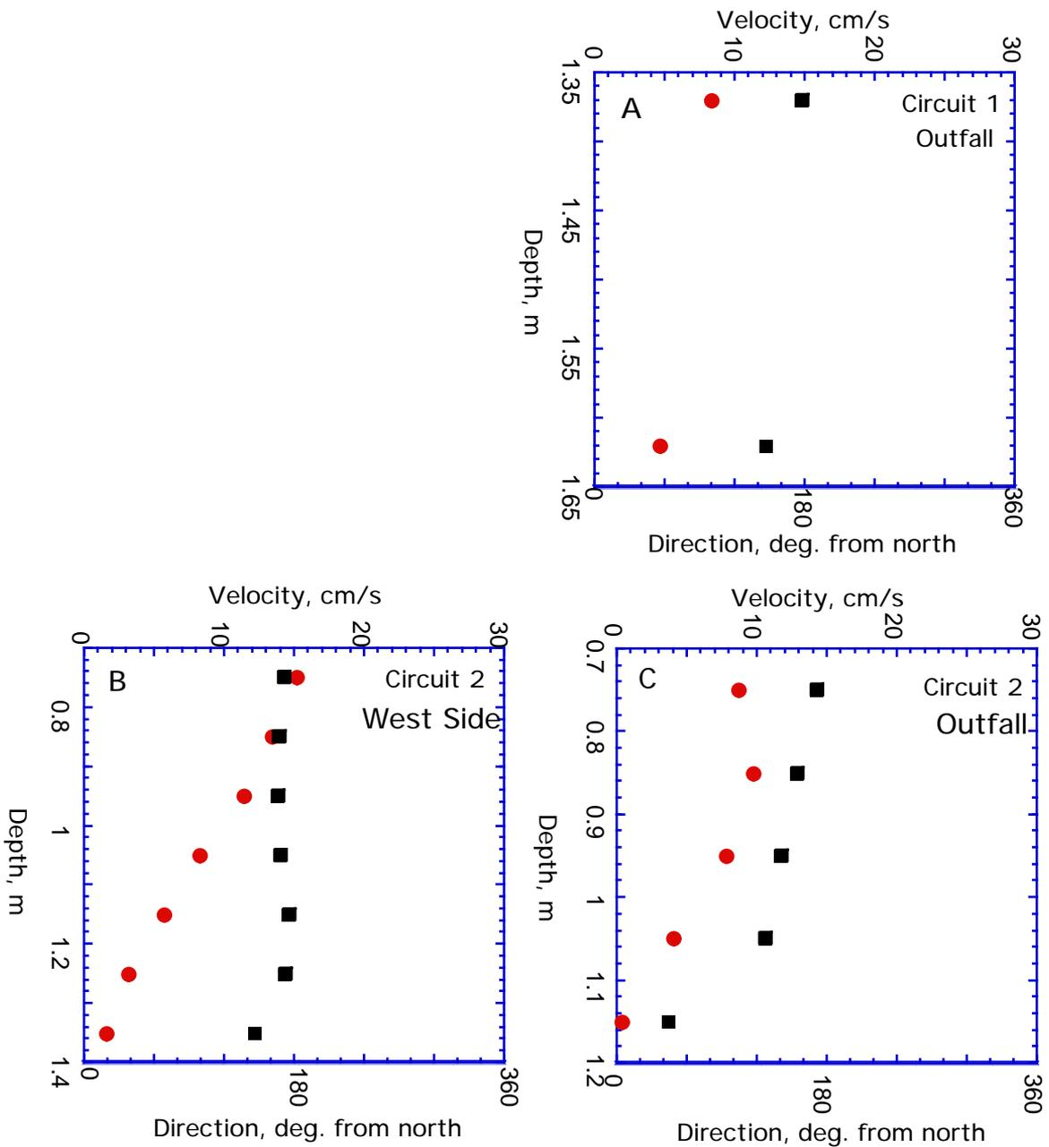
Figure 28: Velocity profiles obtained for transect 2 from times series data collection performed outside the channel, within the eastern (outfall side) and western portions of the Seekonk River. Shown are velocity magnitude (circles) and direction (squares). Data are from circuit 1 (early ebb) and circuit 2 (mid ebb) stages of the tide.
