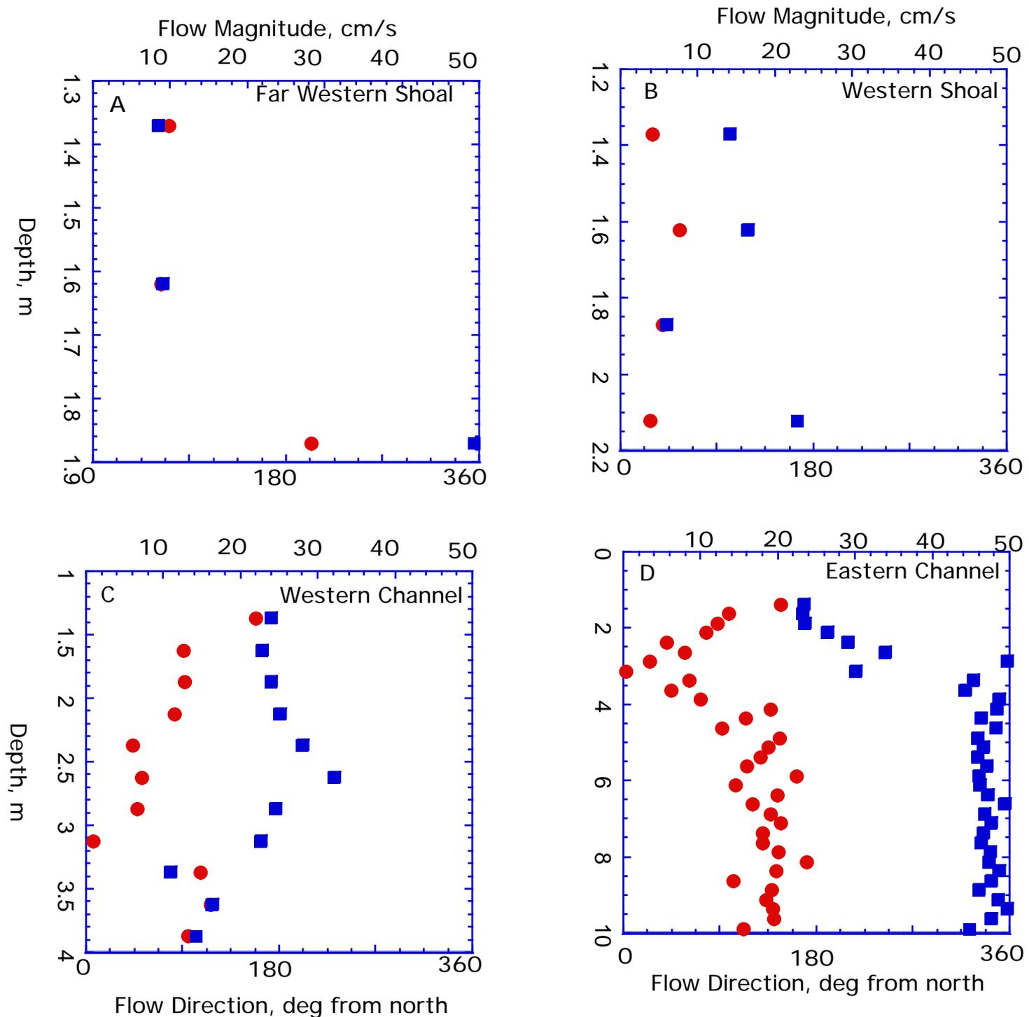
Figure 11: Laterally averaged velocity profiles for subsections of transect line 2, Fields Pt. Data are velocity magnitude (CIRCLES) and direction (SQUARES). The subsections include shallow regions to the west of the channel, and two subsections of the channel. The tidal stage is CIRCUIT 2, or late ebb conditions.
