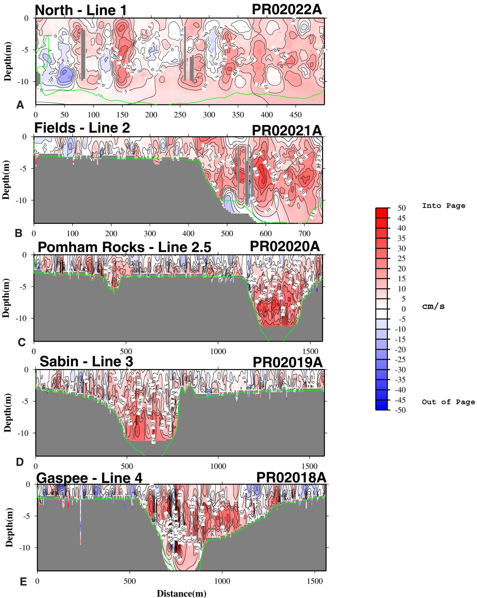
**Figure 5: Circuit 4 (late flood) velocity contours. Velocity vectors are projected normal to the transect line. West is on the left, east is on the right. Red colors are flooding waters, or into the page, blue colors are ebbing waters, or flow out of the page. The green line marks the depth limit of reliable data.**
