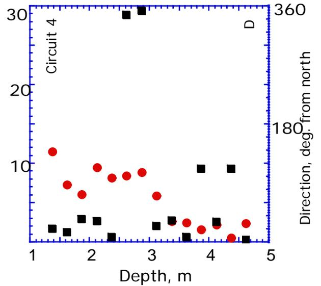
Figure 30 : Velocity profiles obtained for transect 4 by holding position within the channel and collecting data for four minutes. Data have been averaged into a single profile of velocity versus depth. Shown are velocity magnitude (circles) and direction (squares). Data cover tidal stages from early (A), mid(B) and late ebb (C) through to early (D) and mid (E) flood conditions.
