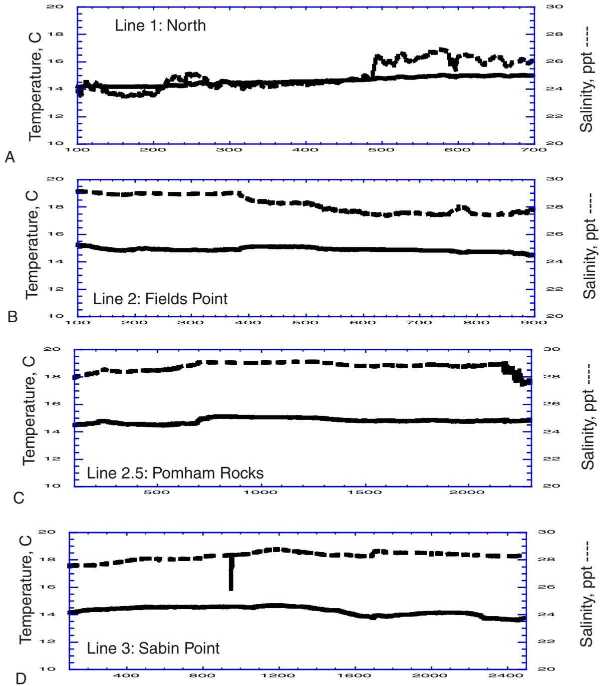
Figure 7: Plots of temperature and salinity measured at the surface versus distance across the estuary for Circuit 2 (late ebb). Orientation is east on the right, west on the left.
