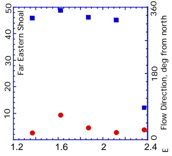
Figure 18: Laterally averaged velocity profiles for subsections of transect line 3, Sabin Pt. Data are velocity magnitude (CIRCLES) and direction (SQUARES). The subsections include shallow regions to the east and west of the channel, and the channel. The tidal stage is CIRCUIT 3, or early flood conditions.
