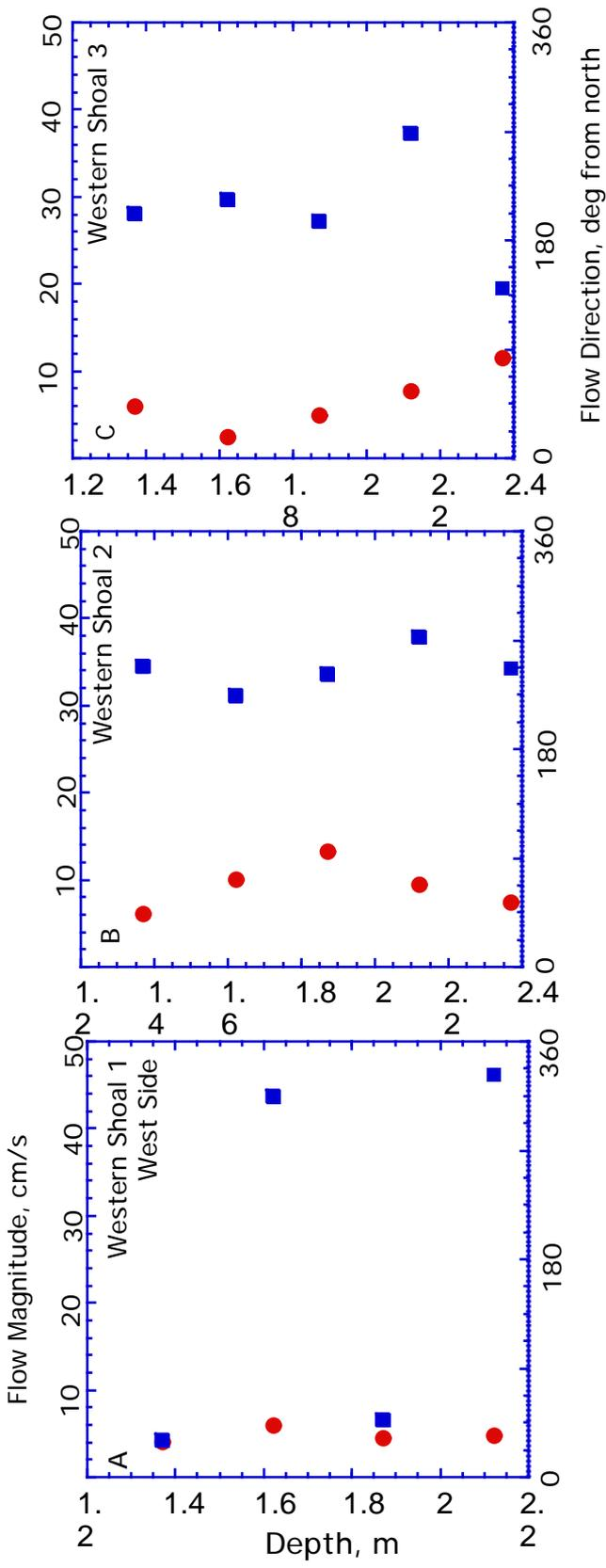
Figure 14: Laterally averaged velocity profiles for subsections of transect line 2.5, Pomham Rocks. Data are velocity magnitude (CIRCLES) and direction (SQUARES). The subsections include shallow regions to the west of the channel, and the channel. Plots A-D are subsections of the shallow region progressing from west to east. The tidal stage is CIRCUIT 2 or late ebb conditions.
