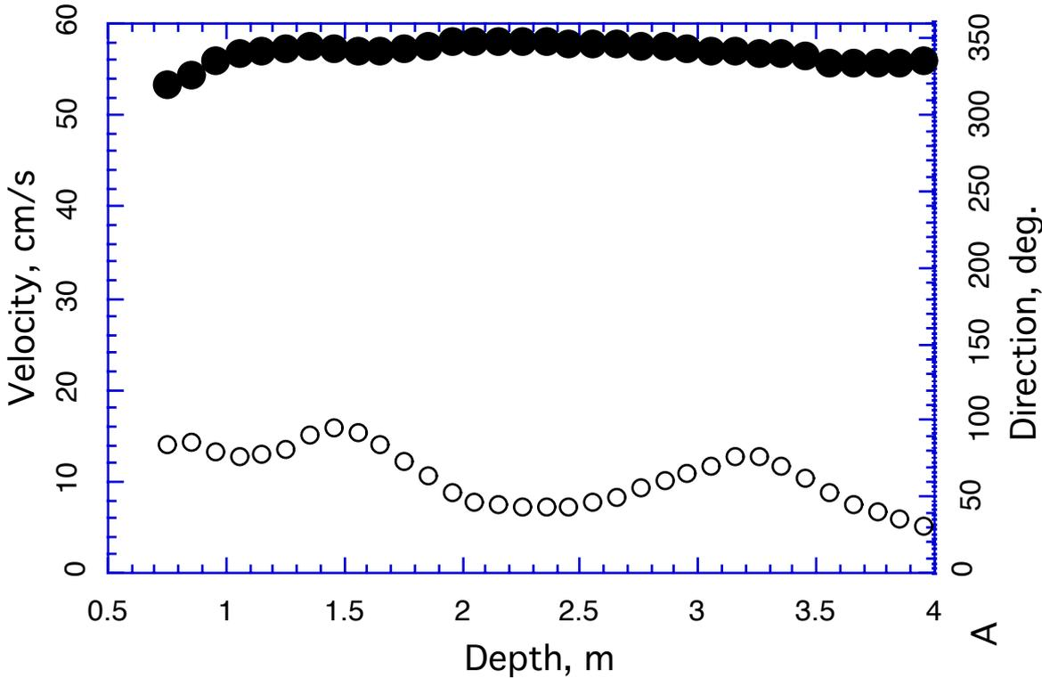
Figure 27: Velocity profiles obtained for transect 1 by holding position within the channel and collecting data for five minutes. Data have been averaged into a single profile of velocity versus depth. Shown are velocity magnitude (open circles) and direction (dark circles).
