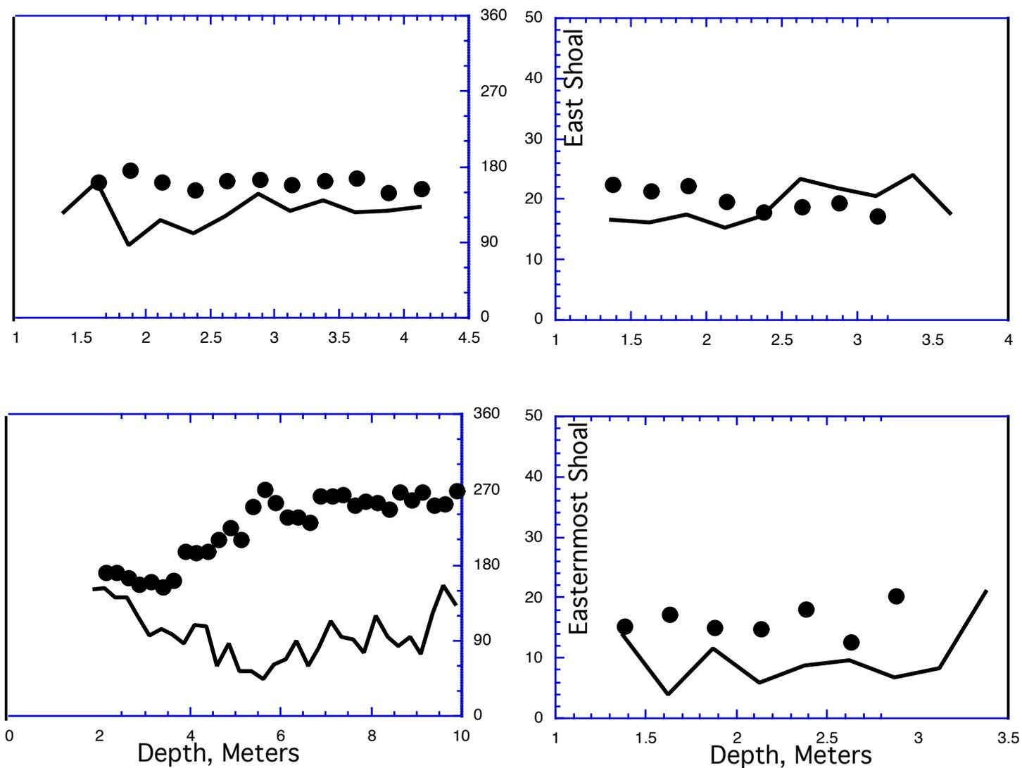
Figure 19: Laterally averaged velocity profiles for distinct sections of transect 3, across Sabin Point. Sections include shoals to the east and west of the channel. The eastern shoal is divided into two sub-sections. Time period is circuit 3, or early ebb conditions. Velocity magnitude(direction)=solid line(dark circles).
