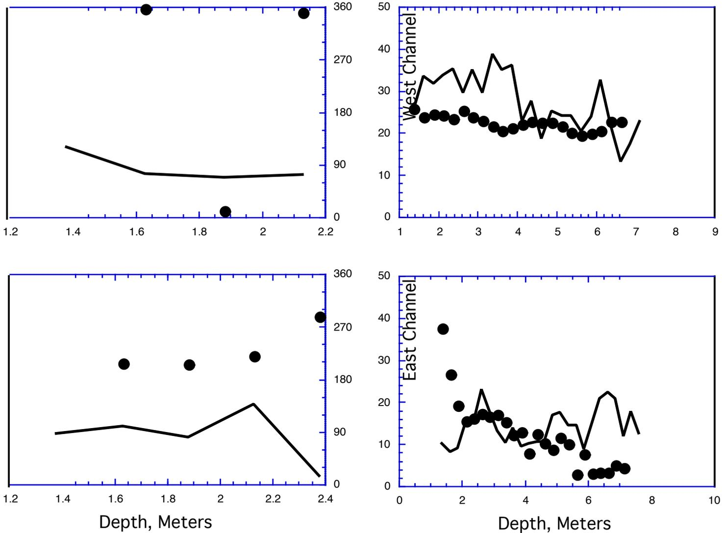
Figure 15: Laterally averaged velocity profiles for distinct sections of transect 2, south of Fields Point. Sections include shallow or shoaling region on the western half of the line and the channel, on the eastern half of the line. Time period is circuit 4, ebb conditions. Velocity magnitude=solid lines. Velocity direction=solid dots.
