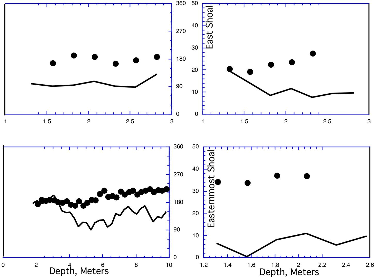
Figure 20: Laterally averaged velocity profiles for distinct sections of transect 3, across Sabin Point. Sections include shoals to the east and west of the channel. The eastern shoal is divided into two sub-sections. Time period is circuit 4, or late ebb conditions. Velocity magnitude(direction)=solid line(dark circles).
