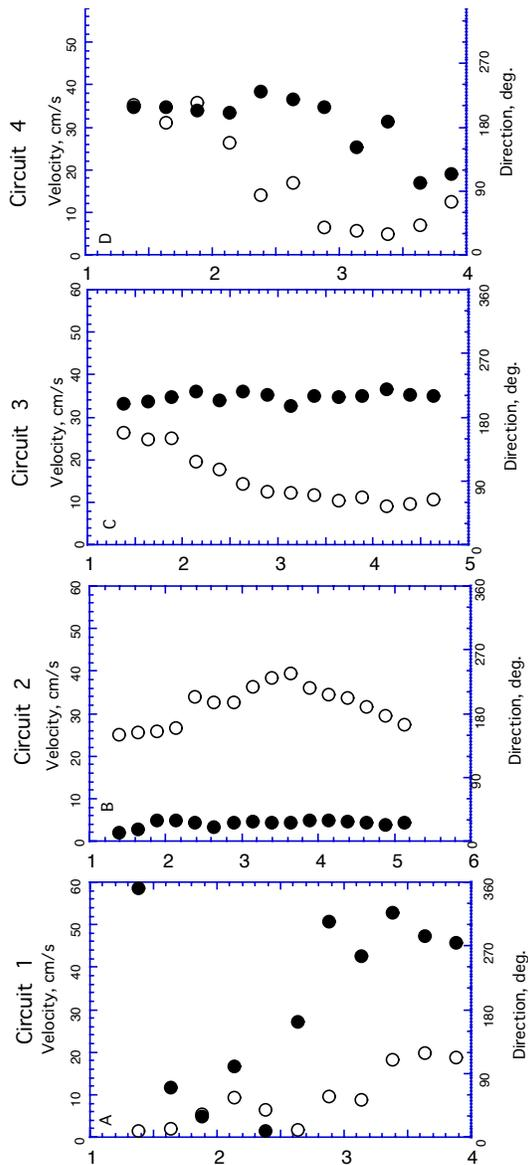
Figure 29: Time averaged velocity profiles collected within the channel for transect 3. Shown are velocity magnitude (open circles) and direction (dark circles).
