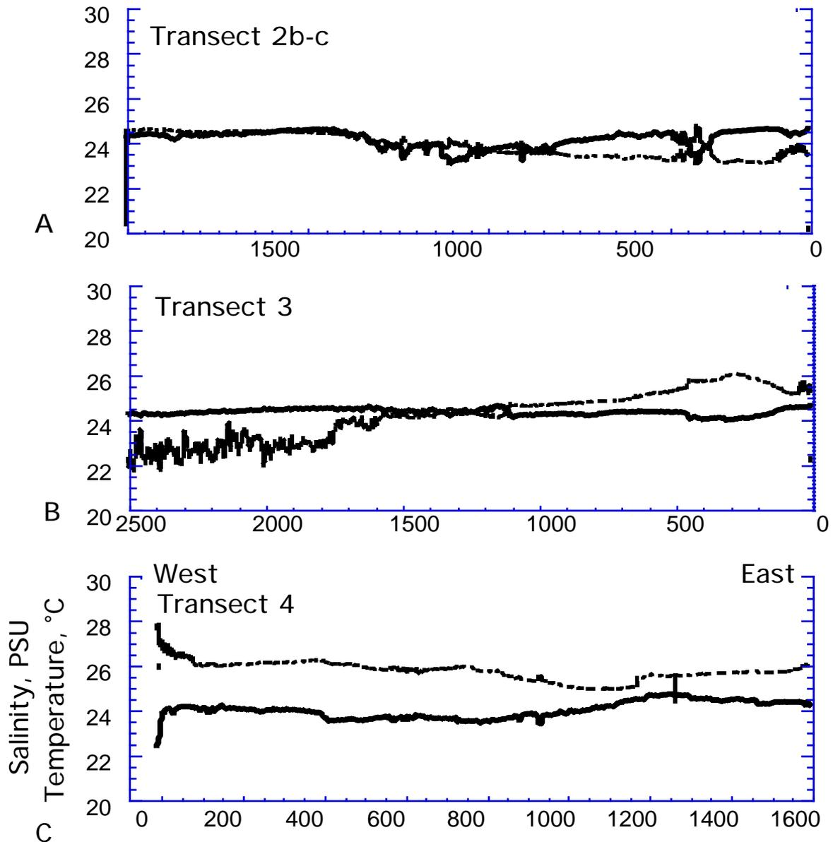
Figure 11: Plots of salinity (dashed line) and temperature (solid) versus distance across the Providence River for circuit 4. The CTD was towed behind the boat at approximately 1 meter depth. Frames A-C are for transect lines 2-4, respectively. The x-axis is sample number.
