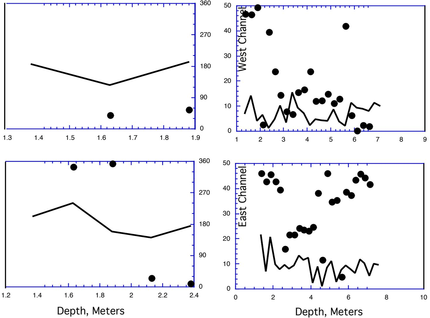
Figure 16: Laterally averaged velocity profiles for distinct sections of transect 2, south of Fields Point. Sections include shallow or shoaling region on the western half of the line and the channel, on the eastern half of the line. Time period is circuit 5, transition from ebb to flood. Velocity magnitude=solid line. Velocity direction=solid dots.
