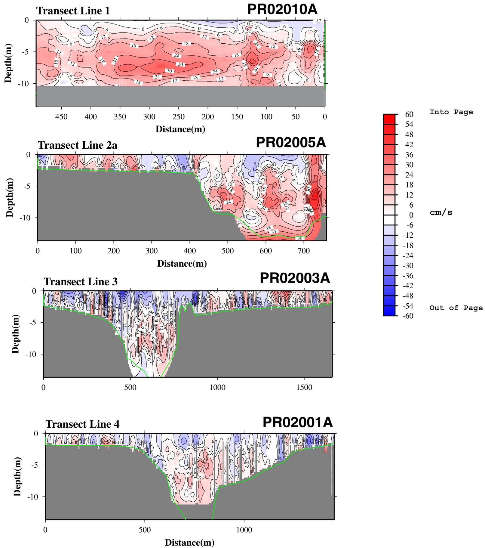
Figure 2: Velocity contour plots for circuit 1, early flood conditions. Orientation is looking north, such that west is to the left and east is to the right. Red colors are flow into the page or flooding waters, blue colors represent flow out of the page, or ebbing water.
