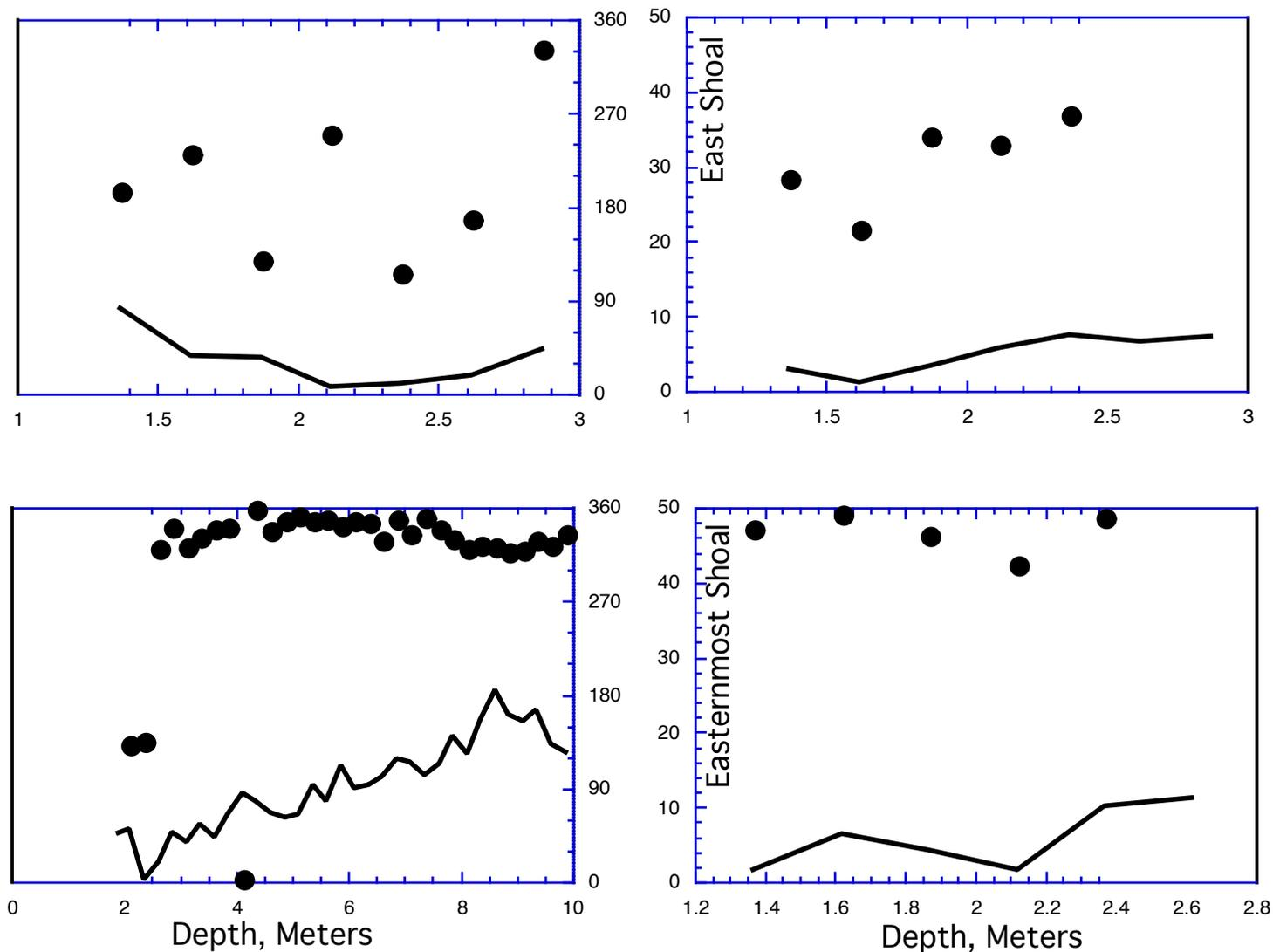
Figure 17: Laterally averaged velocity profiles for distinct sections of transect 3, across Sabin Point. Sections include shoals to the east and west of the channel. The eastern shoal is divided into two sub-sections. Time period is circuit 1, or early flood conditions. Velocity magnitude(direction) = solid lines (dark circles).
