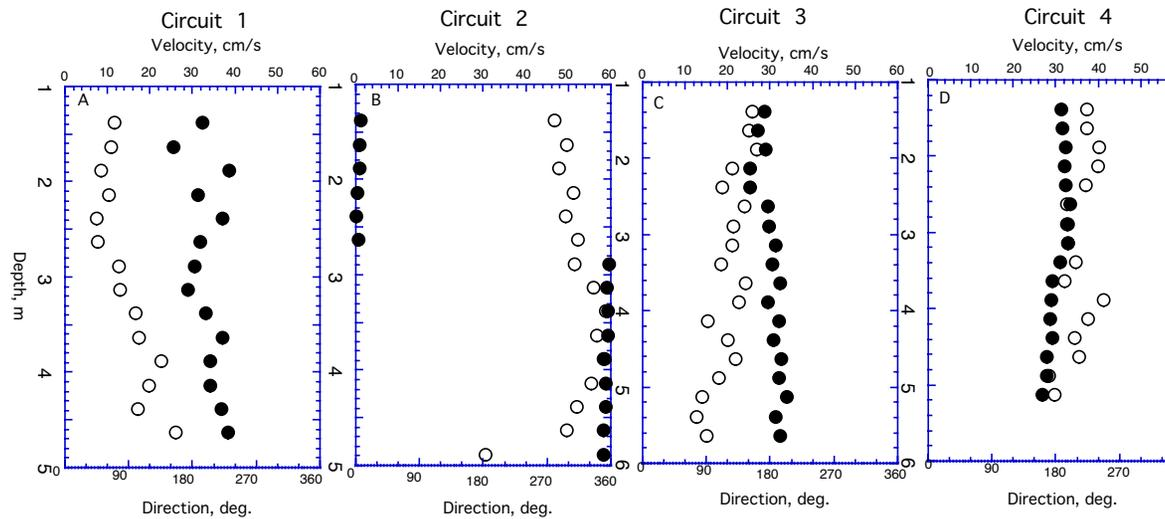
Figure 30: Time averaged velocity profiles collected within the channel for transect 4. Shown are velocity magnitude (open circles) and direction (dark circles).
