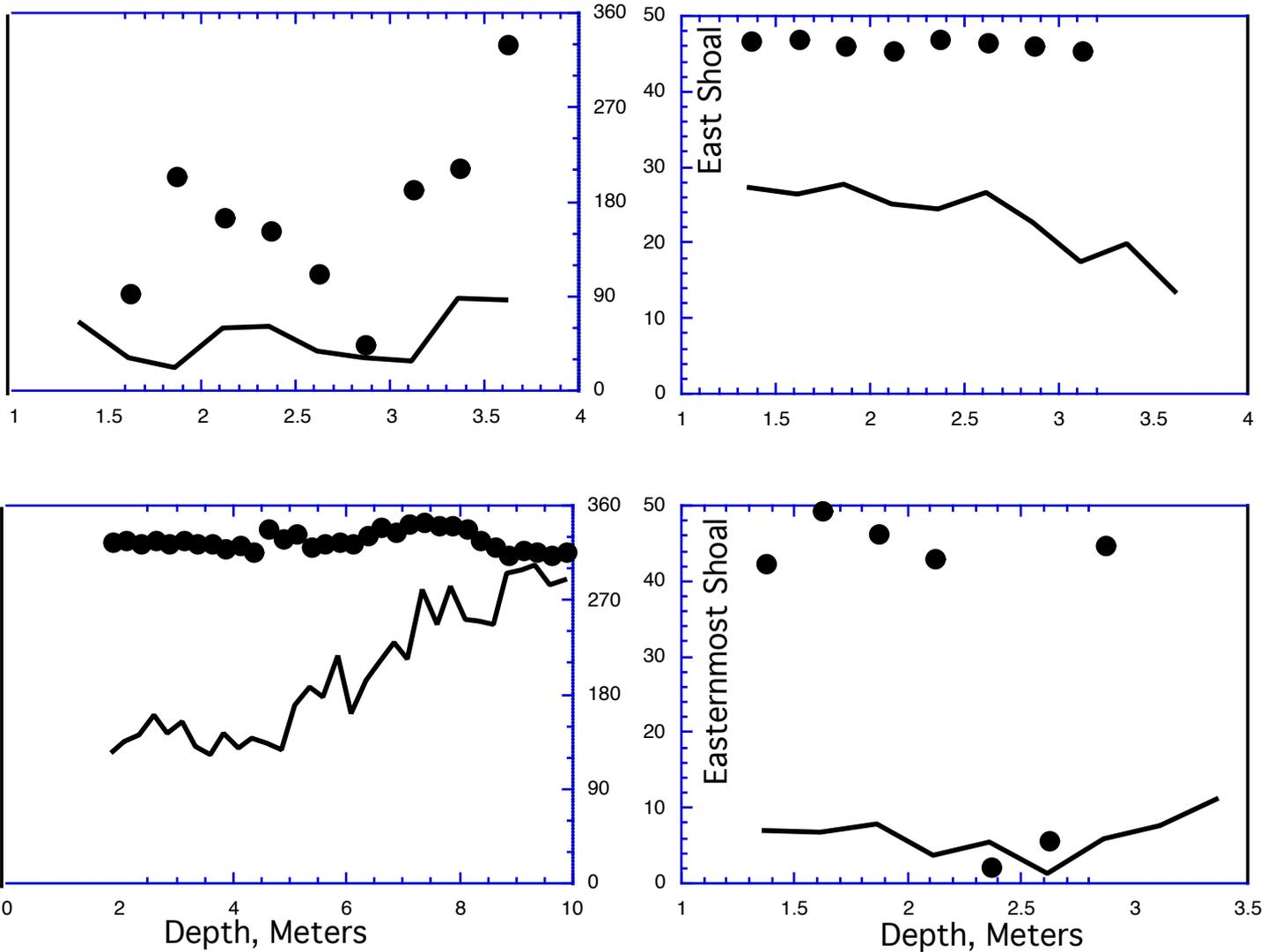
Figure 18: Laterally averaged velocity profiles for distinct sections of transect 3, across Sabin Point. Sections include shoals to the east and west of the channel. The eastern shoal is divided into two sub-sections. Time period is circuit 2, or mid-late flood conditions. Velocity magnitude(direction)=solid lines(dark circles).
