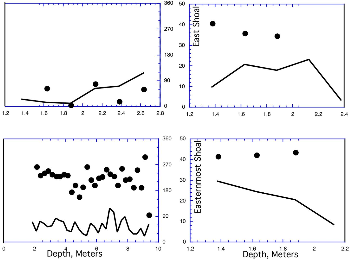
Figure 21: Laterally averaged velocity profiles for distinct sections of transect 3, across Sabin Point. Sections include shoals to the east and west of the channel. The eastern shoal is divided into two sub-sections. Time period is circuit 5, or the transition from ebb to flood conditions. Velocity magnitude(direction)=solid line(dark circles).
