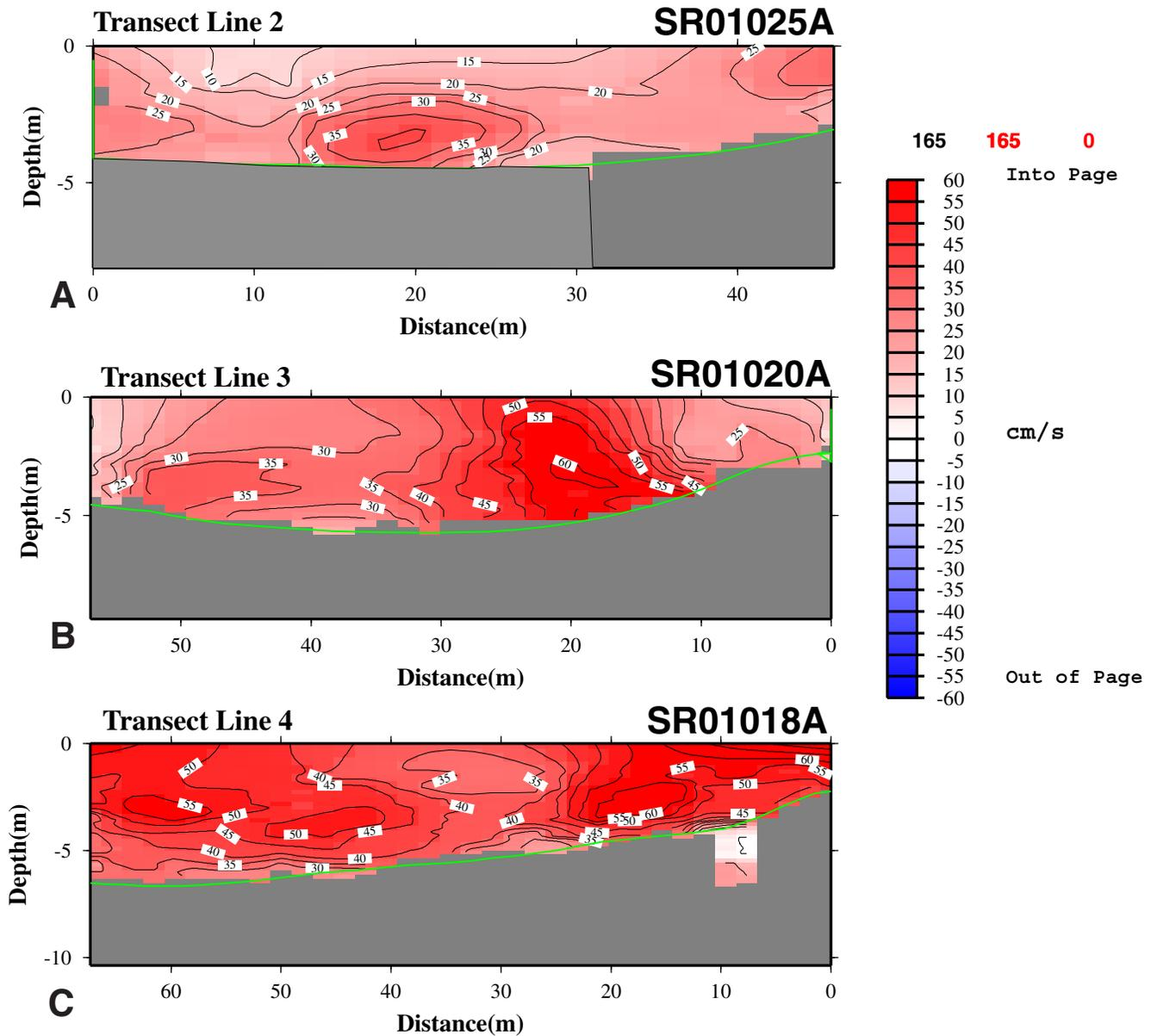
Figure 24: Contour plots for velocity component projected normal to the transect line for data collected on circuit 2, or flood conditions. A: Transect 2, B: Transect 3 and C: Transect 4. Because of low water, lines are only driven within the channel. Strongest flood velocities are recorded on the eastern sides of the channel for lines 3 and 4.
