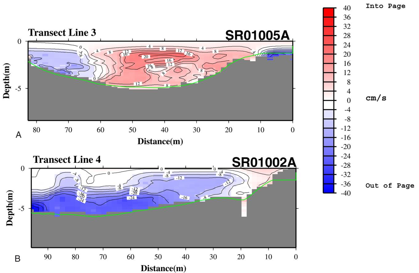
Figure 23: Contours of velocity projected normal to the transect line for circuit 1. Transect lines are number 3 (A) and 4 (B). Transect 4 is sampled earlier and only a small fraction of the cross section shows flooding water, along the eastern side. The river extended beyond this point but was too shallow to be sampled. The majority of the cross section at line 3 is flooding when roughly 1 hour later. The western side which could be sampled is still ebbing.
